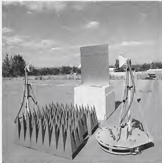
Scattering object testing at NIST OATS facility
